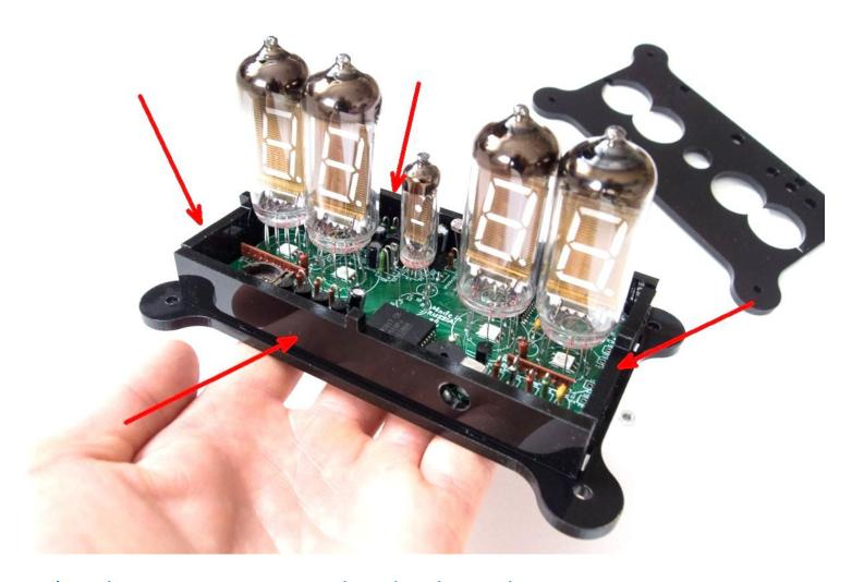
25) At last, insert top panel and tighten the nuts.
