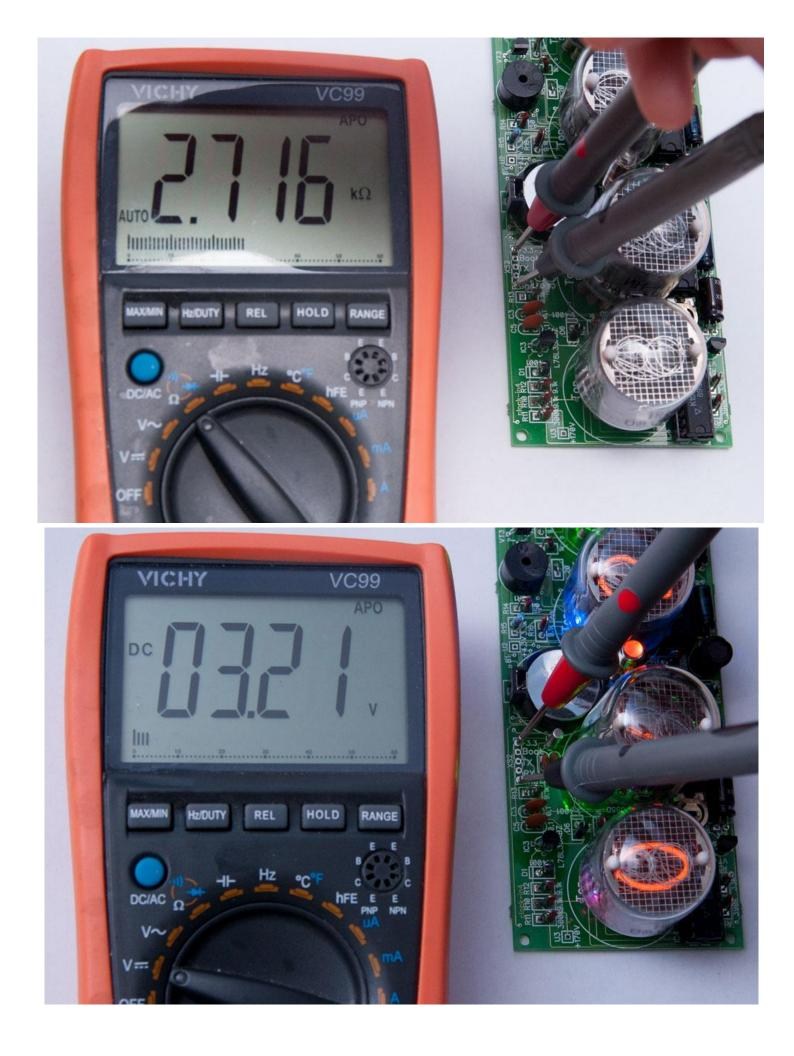
21) And now check high voltage on U3 pad. It should be ~160-170V. Use R6 potentiometer for adjusting.
