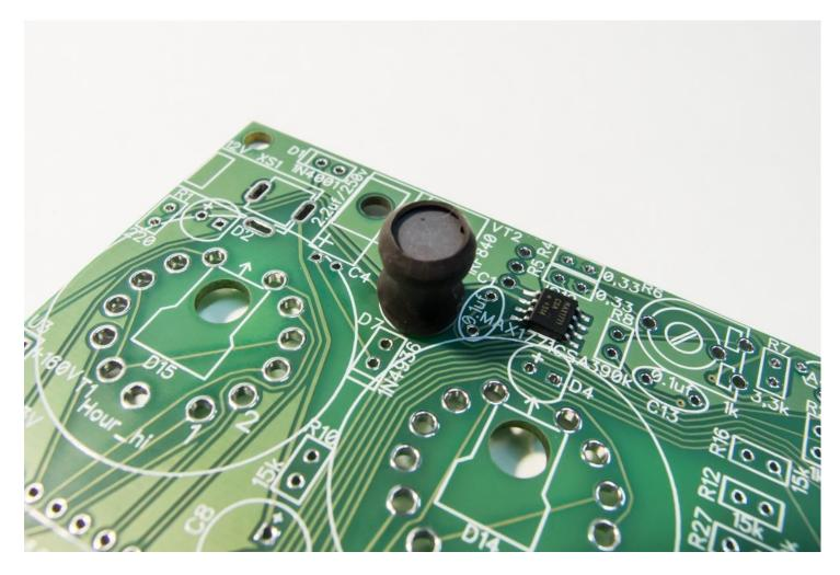
15) Place 2 INS-1 tubes. See the glass dot on INS tube; it should be placed to '+' on PCB.
