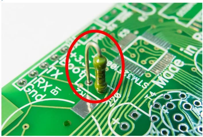
3) Place photoresistor. Make height of photoresistor equal buttons height.
