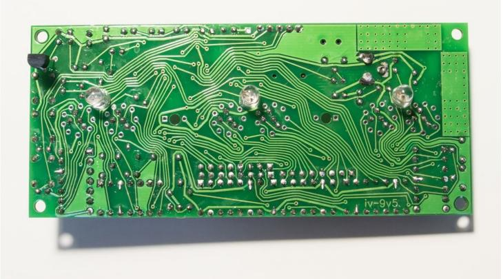
16) Prepare and install all IV-9 tubes. You can see that pins of tubes cuts spiral already. The longest pin – first pin:
