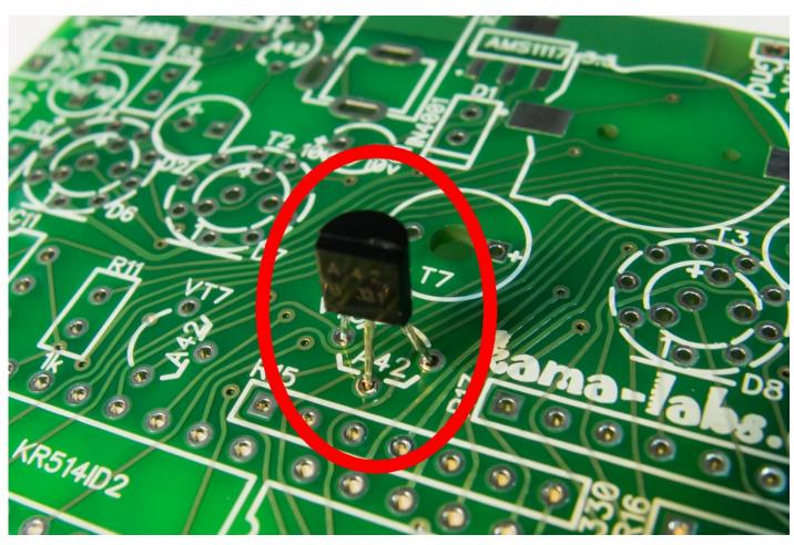
IC11 – temperature sensor and should place on BOTTOM side of PCB:
