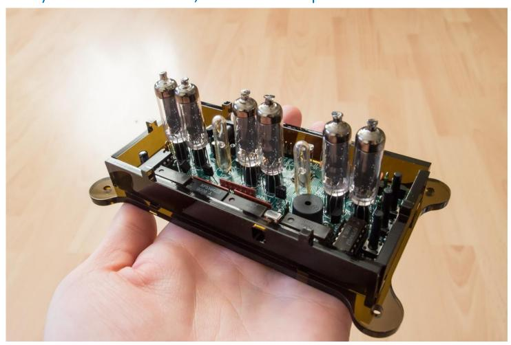
23) At last, insert top panel and tighten the nuts.
