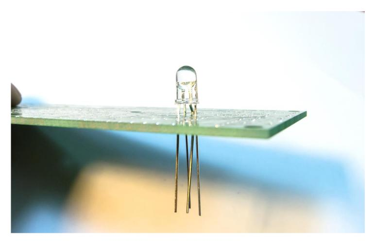
13) Prepare and install AUTO leds. This LEDs should be installed on BOTTOM side of PCB:
