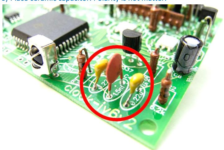
7) Place all transistors and IC5 according marking on PCB:
