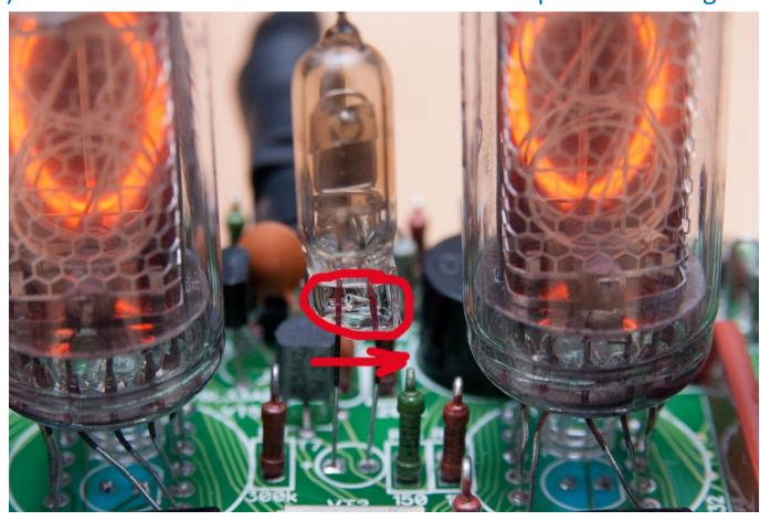
18) Now check the resistance between GND (U7) and +3.3V(U2) pads again. It is should be ~3kOhm. However, not less than 1 kOhm.
