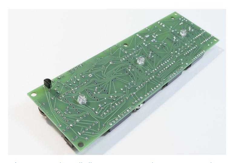
16) Prepare and install all IN-14 or IN-8-2 tubes. You can see that pins of tubes cuts spiral already. The longest pin – first pin:
