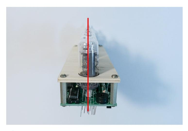
17) Place two IN-3 tubes. Arrow on tube must point to the right:
