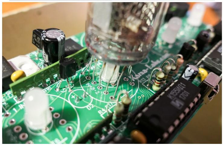
See next photo. For IN-14 tubes, I did make red selection for show first pin on PCB. For IN-8 tubes, I used blue selection. Therefore, the longest pin of tube IN-14 tube should be insert to the 1 hole. First pin of IN-8 tube to the second hole.
