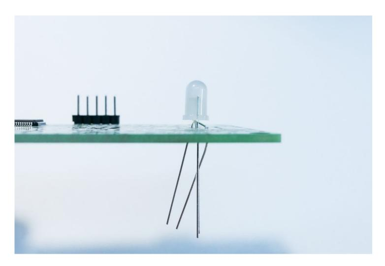
13) Prepare and install AUTO leds. This LEDs can be placed on both sides of PCB also:
