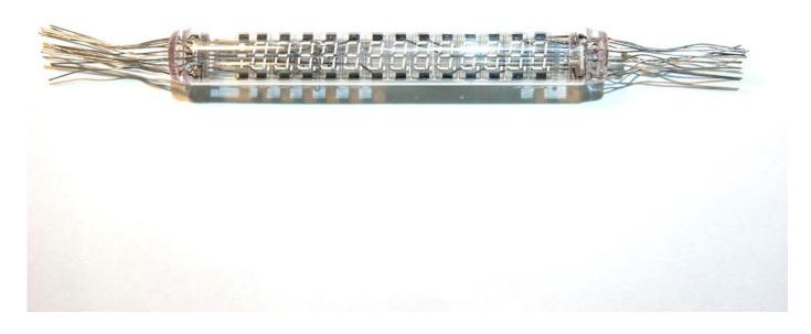
You can see that I already cut pins by spiral. The first pin of tube – the longest pin (on both sides of tube).
