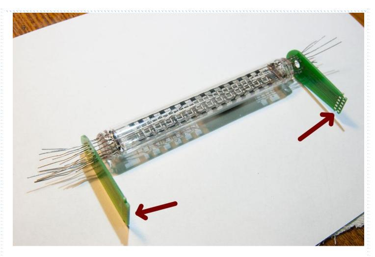
11) Make side PCBs vertically and solder to main PCB on top and bottom sides.
