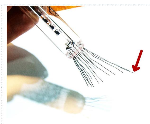
10) Now, insert pins into holes of small PCBs. The first pin on PCBs marks as "1". The pads on PCB should 'look' inside.
