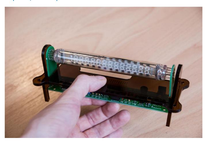
4) Insert legs of side panels into holes on bottom plastic part:
