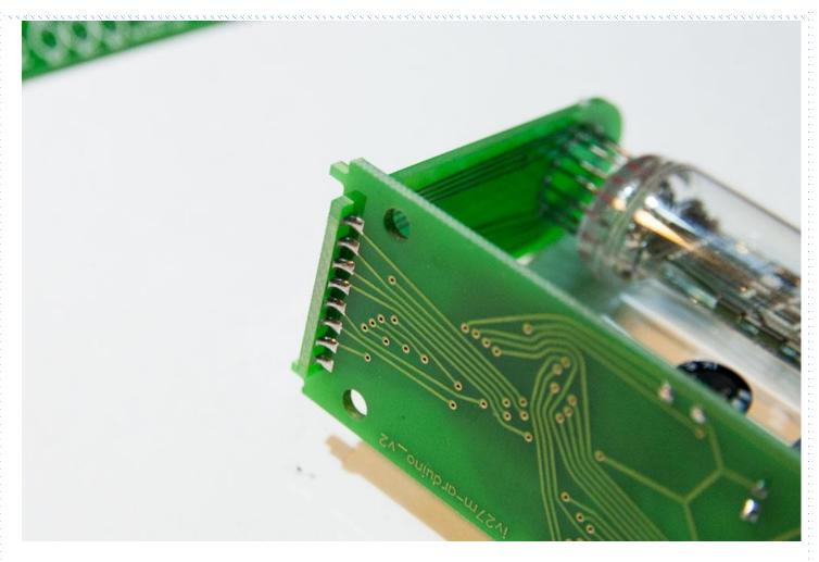
12) At last, you can solder all pins of IV-27 tube to side PCBs.
