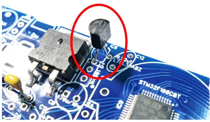
IC11– temperature sensor should place on BOTTOM side of PCB:
