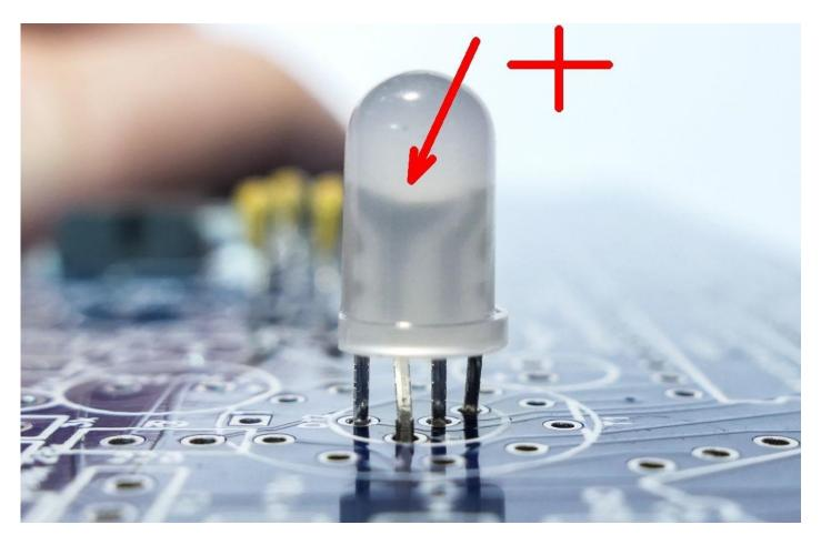
15) Prepare and install AUTO leds. This LEDs should be installed on BOTTOM side of PCB:
