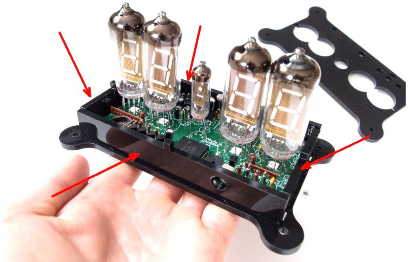
25) At last, insert top panel and tighten the nuts.
