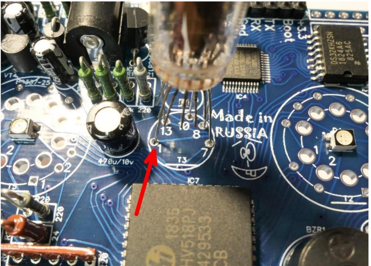
20) Now check the resistance between GND and +3.3V pins of XS2 again. It should be  $\sim 3\text{k}\Omega$ . However, not lower  $1\text{k}\Omega$ .
