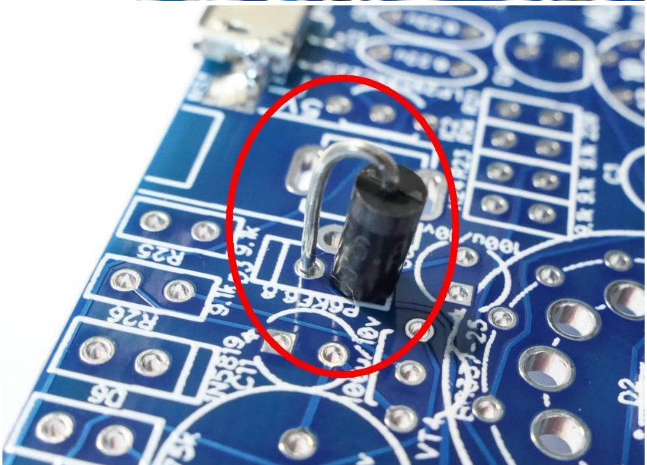
4) Place all electrolytic capacitors. Be careful with polarity!
