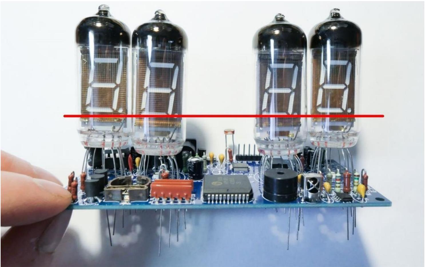
Use wooden fixture to align tubes in straight line.
